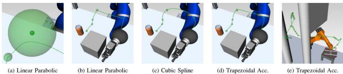
**Figure 4: Trajectories for Various Interpolation Models on Path Designing Use Cases for (a)–(d) a Kuka LWR Next to a Table with a Parallel Gripper and (e) a Kuka KR60-3 Next to a Wall and 3 Columns with a Vacuum Gripper.**
