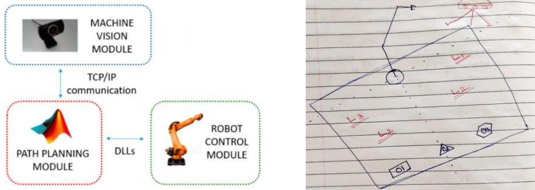
**Figure 1: Overview of the Proposed System, Experimental Diagram of Work Cell.**
